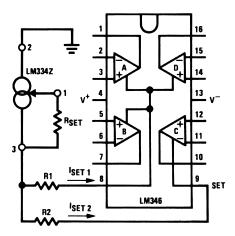
$$\frac{I_{SET1}}{I_{SET2}} = \frac{R2}{R1}, I_{SET1} + I_{SET2} = \frac{67.7 \text{ mV}}{R_{SET}}$$
