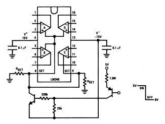
• By pulling the SET pin(s) to V<sup>-</sup> the op amp(s) shuts down and its output goes to a high impedance state. According to this property, the LM346 can be used as a very low speed analog switch.
