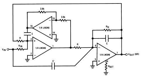
Figure 36. A 3-Amplifier Notch Filter (or Elliptic Filter Building Block)
