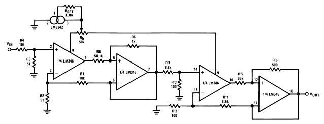
Ex:  $f_c = 20 \text{ kHz}$ ,  $H_o$  (gain of the filter) = 1,  $Q_{01} = 0.541$ ,  $Q_{o2} = 1.306$ .
