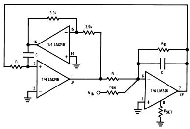
• If resistive biasing is used to set the LM346 performance, the  $Q_o$  of this filter building block is nearly insensitive to the op amp's GBW product temperature drift; it has also better noise performance than the state variable filter.
