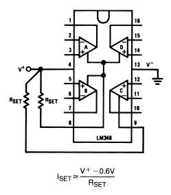
Figure 31. Single (Positive) Supply Biasing
