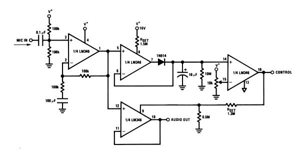
Figure 41. Voice Activated Switch and Amplifier
