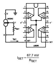
• The LM334 provides an I<sub>SET</sub> directly proportional to absolute temperature. This cancels the slight GBW product Temperature coefficient of the LM346.
