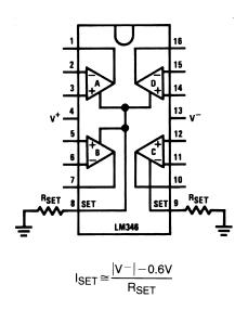
Figure 30. Dual Supply or Negative Supply Blasing
