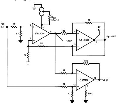
Figure 37. Capacitorless Active Filters (Basic Circuit)
