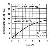
Figure 26. Output Current Limit vs I<sub>SET</sub>
