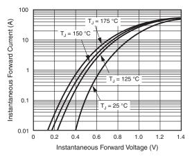
Fig. 3 - Typical Instanteous Forward Characteristics
