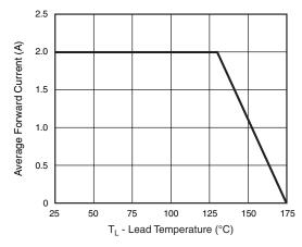
Fig. 1 - Forward Current Derating Curve
