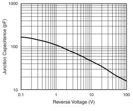
Fig. 5 - Typical Junction Capacitance
