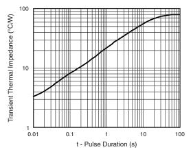
Fig. 6 - Typical Transient Thermal Impedance Per Leg
