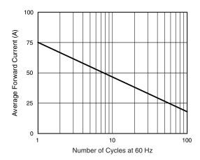
Fig. 2 - Max Non-Repetitive Peak Forward Surge Current
