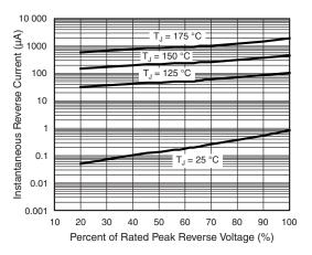
Fig. 4 - Typical Reverse Characteristics
