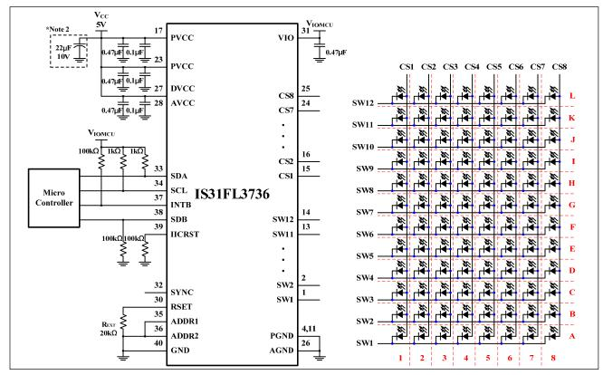
Figure 1 Typical Application Circuit (12×8)
