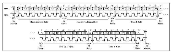
Figure 7 Writing to IS31FL3736 (Automatic address increment)
