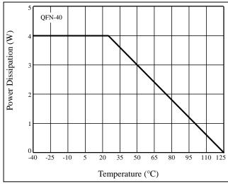
Figure 17 Dissipation Curve
