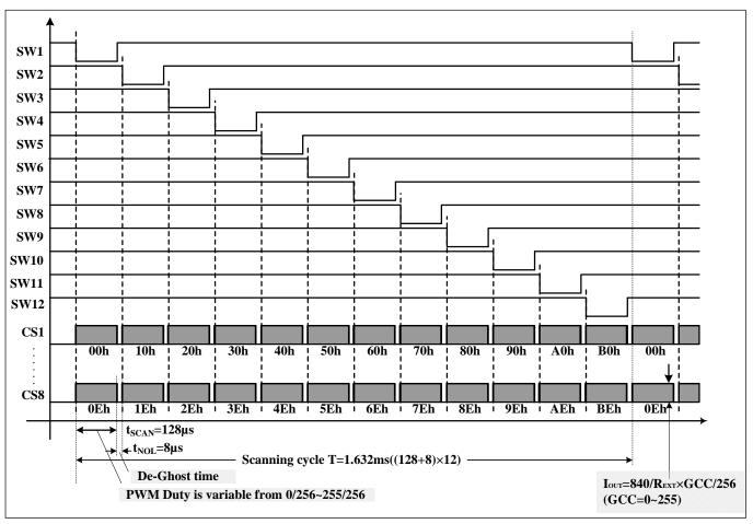
Figure 12 Scanning Timing
