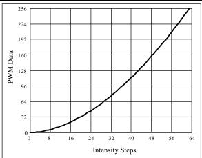
Figure 14 Gamma Correction (64 Steps)
