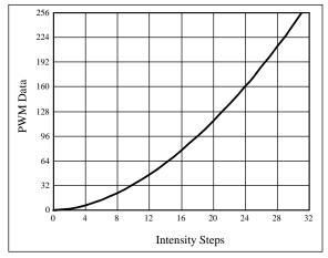
Figure 13 Gamma Correction (32 Steps)
