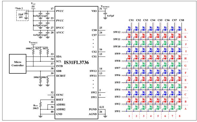
Figure 2 Typical Application Circuit (RGB)
