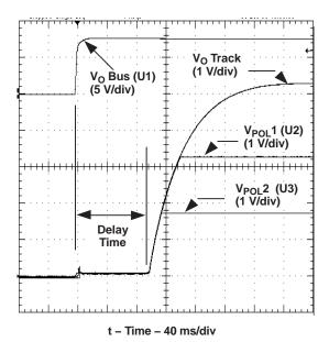
Figure 9. AutoTrack™ Control Waveform
