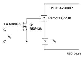
Figure 6. Recommended Control for Remote On/Off Input
