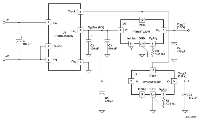
Figure 8. Power-Up Sequencing Using AutoTrack™ Control
