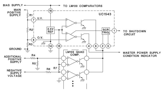
Figure 8. Sensing Multiple Supply Voltages
