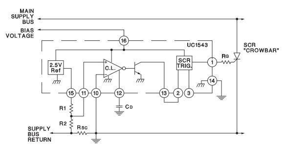
Figure 10. Overcurrent Shutdown
