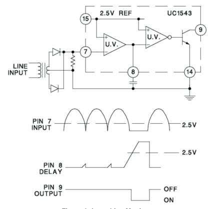
Figure 9. Input Line Monitor
