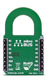
**Secure click** carries the ATECC508A cryptographic coprocessor with secure hardware-based key storage. The click is designed to run on either 3.3V or 5V power supply. It communicates with the target microcontroller over I2C interface.
