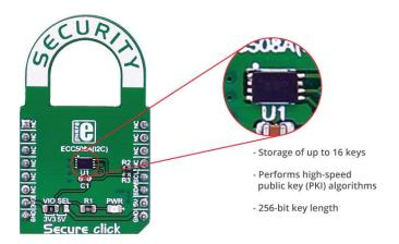
The ATECC508A includes an EEPROM array which **can be used for storage of up to 16 keys**, certificates, miscellaneous read/write, read-only or secret data, consumption logging, and security configurations. Access to the various sections of memory can be restricted in a variety of ways and then the configuration can be locked to prevent changes.
