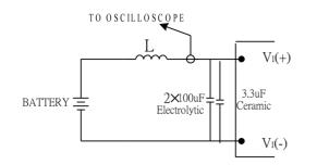
Note: Input reflected-ripple current is measured with a simulated source inductance. Current is measured at the input of the module.
