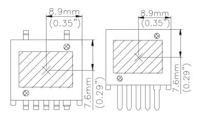
**Figure 25:** Temperature measurement location \* The allowed maximum hot spot temperature is defined at 125 C.
