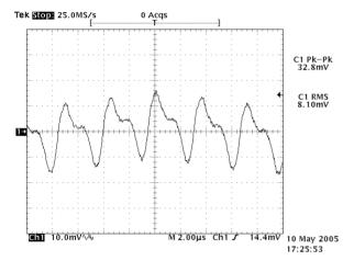
Figure 3: Output ripple & noise at 36Vin, 8.0V/3A out
