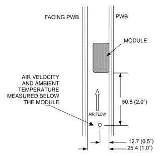
**Note:** Figure dimensions are in millimeters and (inches) Figure 24: Wind tunnel test setup
