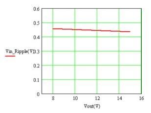
**Figure 18:** Input ripple voltage for various output models, Io = 3A (Cin =2x100uF electrolytic capacitors 1x3.3uF ceramic capacitors at the input)
