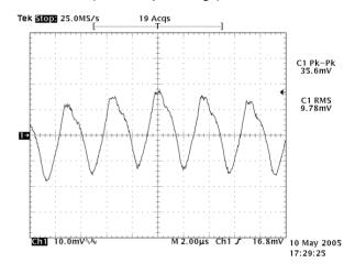
Figure 4: Output ripple & noise at 36Vin, 15.0V/3A out
