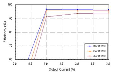
Figure 2: Converter efficiency vs. output current (15.0V output voltage)
