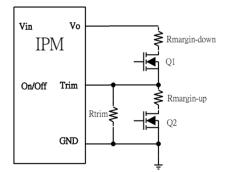
Figure 23: Circuit configuration for output voltage margining
