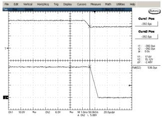
Figure 8: Power off waveform 24vin, 15.0V/3A out with application of Vin
