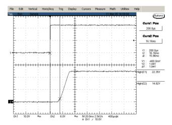
*Figure 12: Turn on delay at 24vin, 15.0V/3A out with application of Vin*
