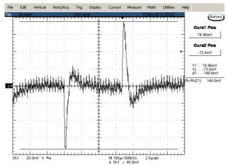
**Figure 13:** Typical transient response to step load change at 0.5A/µS from 100% to 50% of lo, max at 24Vin, 15.0V out (measurement with a 1µF ceramic
