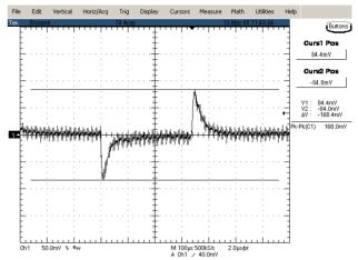
**Figure 14:** Typical transient response to step load change at 0.5A/µS from 50% to 100% of lo, max at36Vin, 6.5V out (measurement with a 1uF ceramic)
