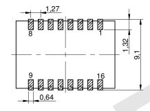
no vias or traces underneath the component Scale - 3:1
