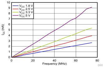
Figure 6. I<sub>CC</sub> vs Frequency
