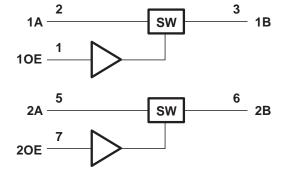
Figure 3. Logic Diagram (Positive Logic)
