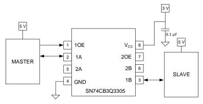
Figure 4. Typical Application of the SN74CB3Q3305
