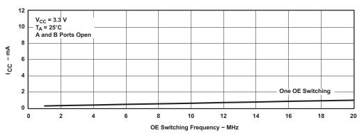
Figure 5. Typical I<sub>CC</sub> vs OE Switching Frequency
