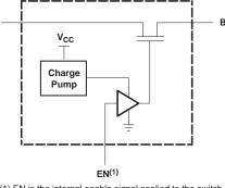
(1) EN is the internal enable signal applied to the switch.
