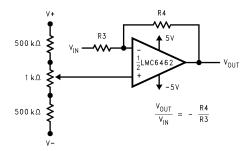
Figure 41. Inverting Configuration Offset Voltage Adjustment
