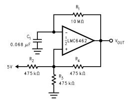
Figure 55. 1 Hz Square-Wave Oscillator
