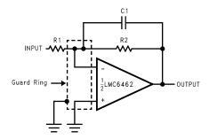
Figure 44. Typical Connections of Guard Rings – Inverting Amplifier
