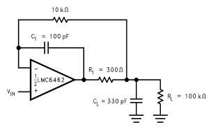
Figure 38. LMC6462 Non-Inverting Amplifier, Compensated to Handle a 300 pF Capacitive and 100 k $\Omega$  Resistive Load
