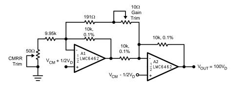
Figure 49. Low-Power Two-Op-Amp Instrumentation Amplifier
