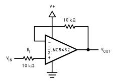
Figure 52. Half-Wave Rectifier with Input Current Protection (R<sub>I</sub>)
