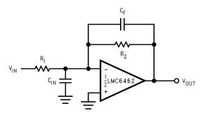
Figure 40. Canceling the Effect of Input Capacitance
