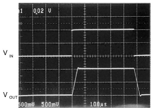
Figure 39. Pulse Response of LMC6462 Circuit in Figure 38
