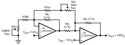
Figure 3. Low-Power Two-Op-Amp Instrumentation Amplifier
