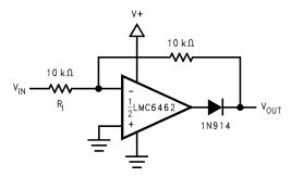
Figure 53. Full-Wave Rectifier with Input Current Protection (R<sub>I</sub>)
