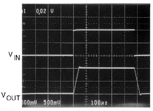
Figure 37. Pulse Response of the LMC6462 Circuit Shown in Figure 36
