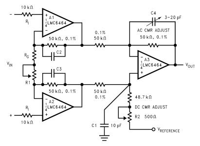
Figure 48. Low Power Three Op-Amp Instrumentation Amplifier
