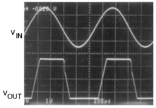
Figure 34. A ±7.5V Input Signal Greatly Exceeds the 3V Supply in Figure 35 Causing No Phase Inversion Due to R<sub>I</sub>
