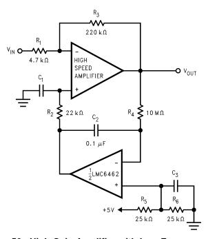
Figure 56. High Gain Amplifier with Low Frequency Null
