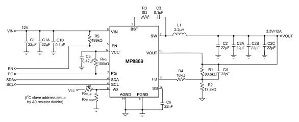
Figure 19:  $V_{IN} = 12V$ ,  $V_{OUT} = 3.3V$ ,  $I_{OUT} = 12A^{(11)}$
