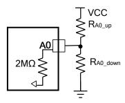
Figure 6: I<sup>2</sup>C Slave Address Selection Set-Up
