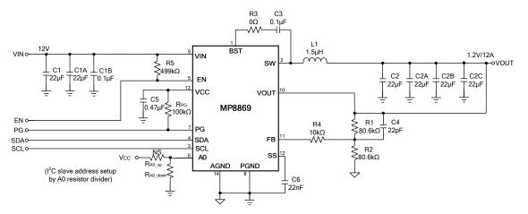
Figure 15: VIN = 12V, VOUT = 1.2V, IOUT = 12A
