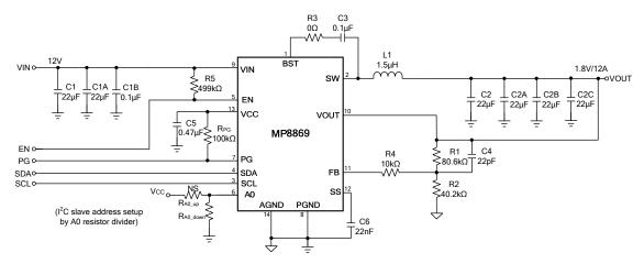
Figure 17:  $V_{IN} = 12V$ ,  $V_{OUT} = 1.8V$ ,  $I_{OUT} = 12A$
