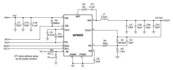
Figure 20:  $V_{IN} = 12V$ ,  $V_{OUT} = 5V$ ,  $I_{OUT} = 12A^{(11)}$
