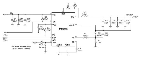
Figure 16: VIN = 12V, VOUT = 1.5V, IOUT = 12A
