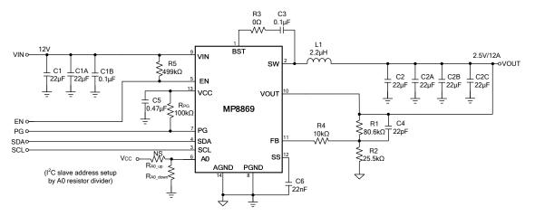
Figure 18: VIN = 12V, VOUT = 2.5V, IOUT = 12A
