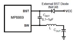
Figure 12: Optional External Bootstrap Diode to Enhance Efficiency
