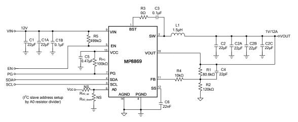
Figure 14: V<sub>IN</sub> = 12V, V<sub>OUT</sub> = 1V, I<sub>OUT</sub> = 12A
