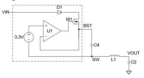
Figure 5: Internal Bootstrap Charging Circuit
