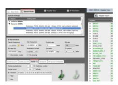
You can now configure the radio, performance tests, export register settings and run link tests with another CC1200 or CC1201 on a SmartRF TrxEB connected to the PC.
