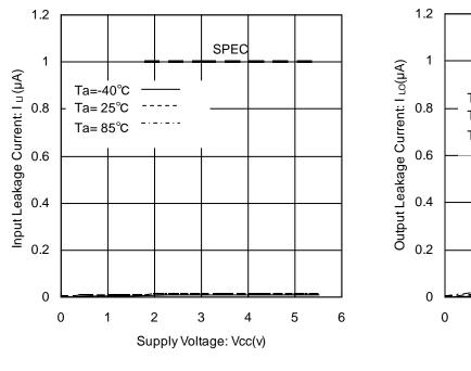
Figure 8. Input Leakage Current vs. Supply Voltage (A2, SCL, WP)
