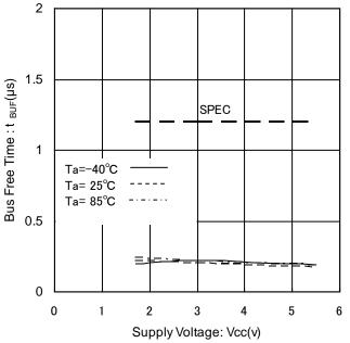
Figure 25. Bus Free Time vs. Supply Voltage
