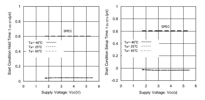
Figure 16. Start Condition Hold Time vs. Supply Voltage
