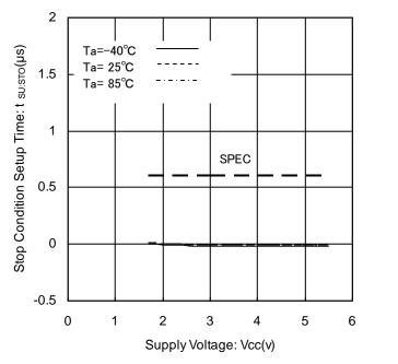
Figure 24. Stop Condition Setup Time vs. Supply Voltage
