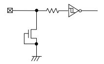
Figure 49. Input Pin Circuit Diagram
