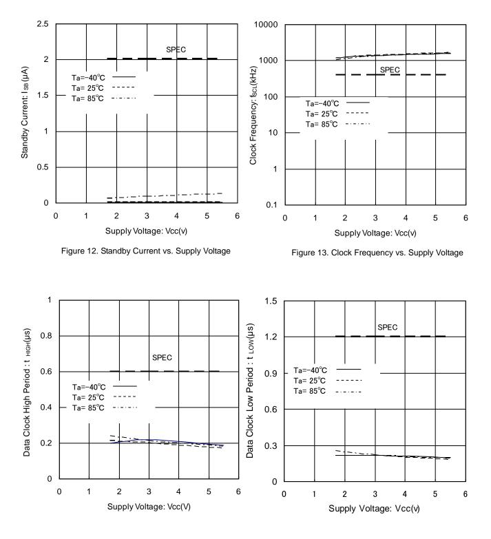
Figure 14. Data Clock High Period vs Supply Voltage
