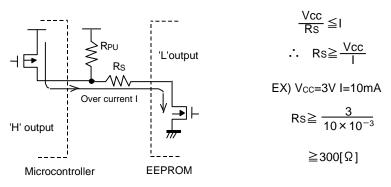
Figure 48. I/O Circuit Diagram
