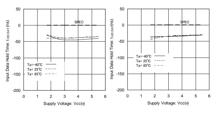
Figure 18. Input Data Hold Time vs. Supply Voltage (HIGH)
