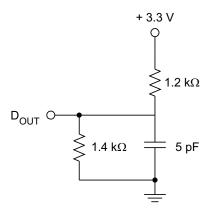
Figure 3. 3.3-V Output Load A
