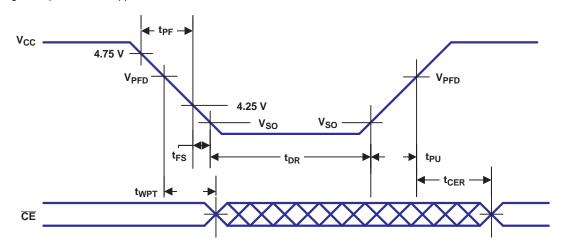
Figure 10. 5-V Power-Down/Power-Up Timing
