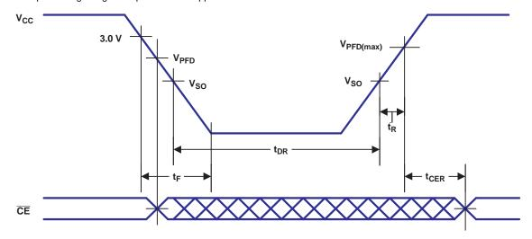
Figure 11. 3.3-V Power-Down/Power-Up Timing
