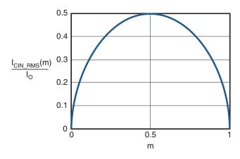
Figure 2. I<sub>CIN</sub> vs. Voltage Conversion Ratio
