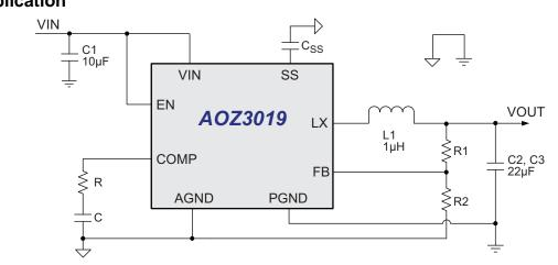
Figure 1. 1.05V, 6A Synchronous Buck Regulator, Fs = 500kHz
