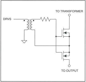
Figure 2. Sampling circuit with two FETs.
