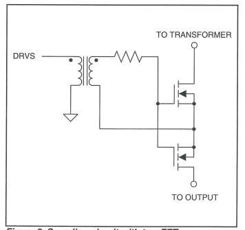
Figure 2. Sampling circuit with two FETs.
