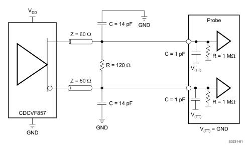
Figure 3. Output Load Test Circuit for Crossing Point
