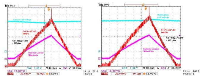
Figure 7-1. Inductor Efficiency
