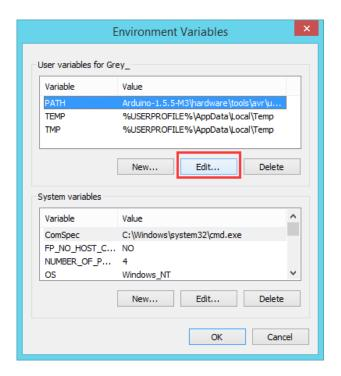
3. Copy the Arduino IDE 1.5.5 (Bluno M3 Version) directory path you downloaded before in to PATH. For example: **C:\Arduino\hardware\tools\avr\utils\bin**. Click **OK**.
