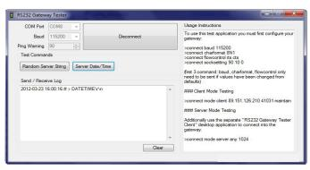
The RS232 Gateway Tester Client responds back with the requested date and time as shown in figure 12 below.
