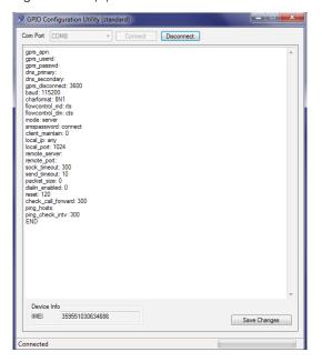
Once the terminal is connected using the serial port, the standard setup parameters will be displayed as shown in figure 2 above.
