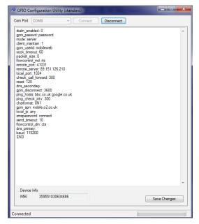
\*The parameters shown in the figure above (baud rate, character formatting, flow control, socksetting) must be configured on the unit by SMS or by using the utility.
