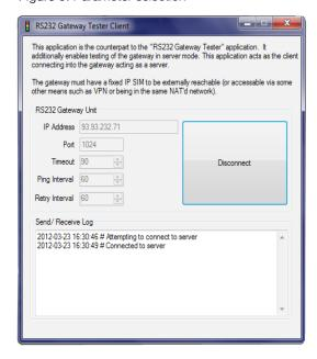
The Client tester will display a prompt as shown in figure 9 above once connected to the LC200 Series server.
