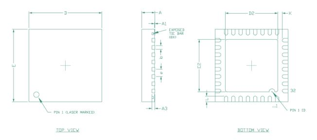
Figure 14-31 Package drawing and mechanical dimensions
