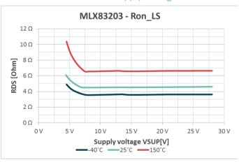
Figure 10-8 MLX83203 Low-side driver FET  $R_{ON}$  resistance vs. supply voltage
