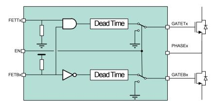
Figure 12-21 Input control logic of the driver stage
