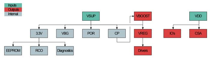
Figure 12-17 Principle organization of the supply system
