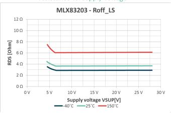
Figure 10-9 MLX83203 Low-side driver FET R<sub>OFF</sub> resistance vs. supply voltage
