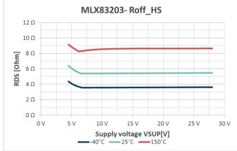
Figure 10-6 MLX83203 High-side driver FET R<sub>ON</sub> resistance vs. supply voltage
