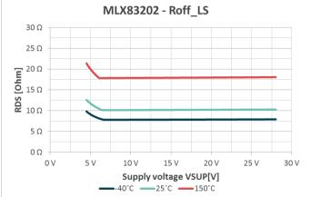
Figure 10-14 MLX83202 Low-side driver FET R<sub>ON</sub> resistance vs. supply voltage
