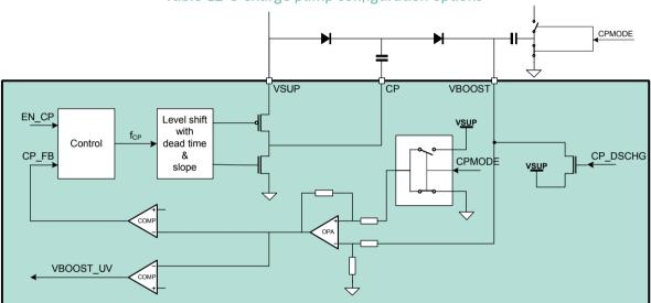
Figure 12-18 Charge pump principle schematic
