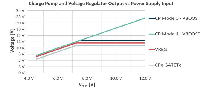
Figure 12-19 Charge pump output and driver supply
