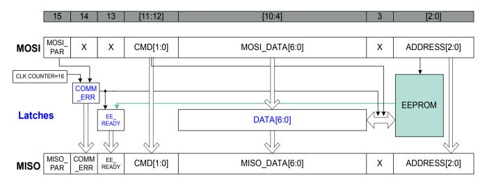
Figure 12-28 MOSI/MISO registers and relation to internal data latches
