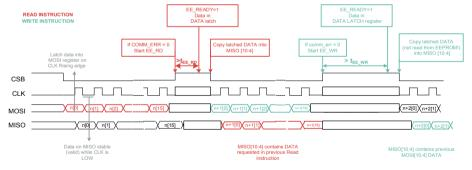
Figure 12-27 SPI Protocol (LSB first)
