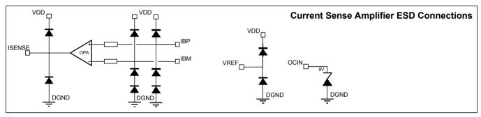
Figure 13-29 Principle Schematic highlighting ESD Connections
