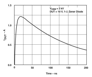
Figure 8. Typical HBM Current Waveform
