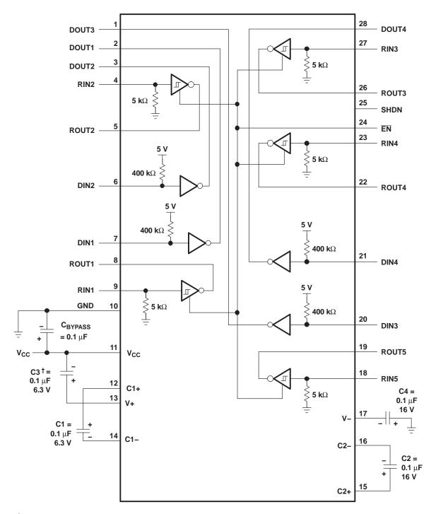
$<sup>^{\</sup>dagger}$  C3 can be connected to  $V_{CC}$  or GND.
