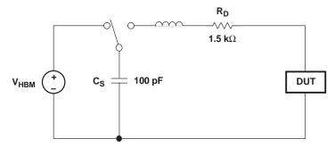
Figure 7. HBM ESD Test Circuit
