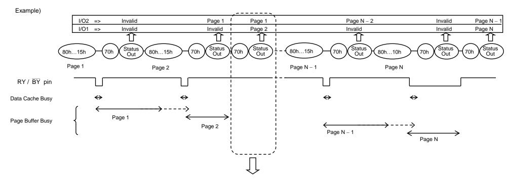
If the Page Buffer Busy returns to Ready before the next 80h command input and Status Read is done during this Ready period, the Status Read provides the Pass/Fail result for Page 2 on I/O1 and the Pass/Fail result for Page1 on I/O2.
