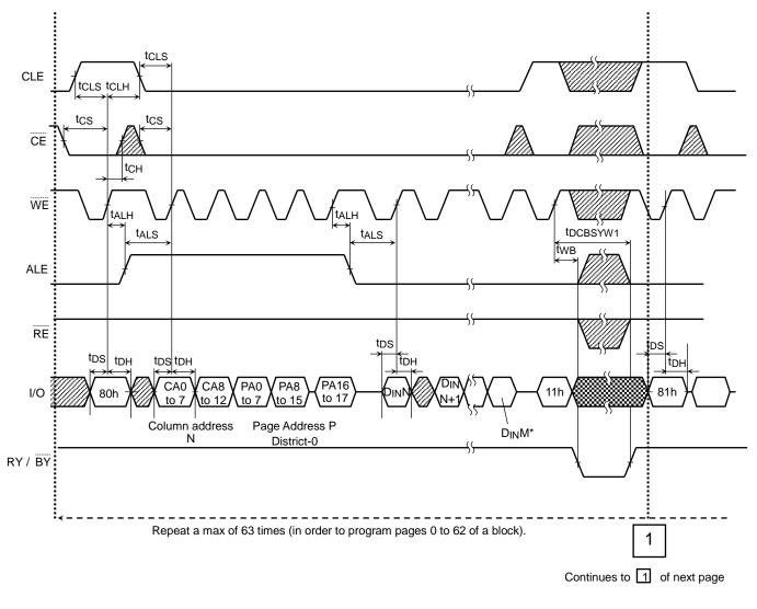
: Do not input data while data is being output.
