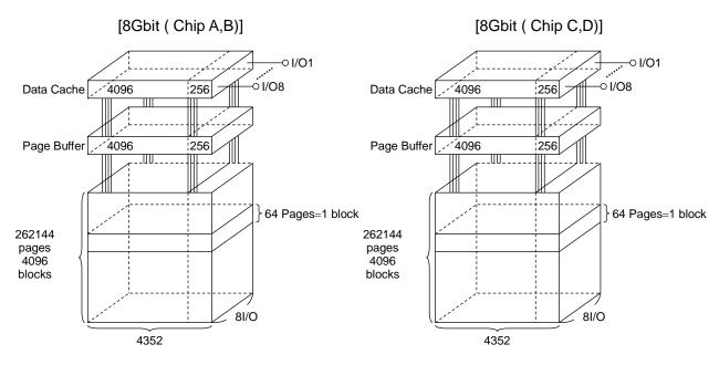
A page consists of 4352 bytes in which 4096 bytes are used for main memory storage and 256 bytes are for redundancy or for other uses.
