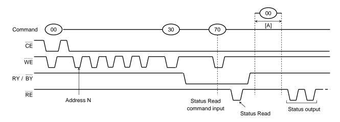
The device status can be read out by inputting the Status Read command "70h" in Read mode. Once the device has been set to Status Read mode by a "70h" command, the device will not return to Read mode unless the Read command "00h" is input during [A]. If the Read command "00h" is input during [A], Status Read mode is reset, and the device returns to Read mode. In this case, data output starts automatically from address N and address input is unnecessary.
