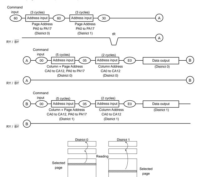
The data transfer operation from the cell array to the Data Cache via Page Buffer starts on the rising edge of  $\overrightarrow{WE}$  in the 30h command input cycle (after the 2 Districts' address information has been latched). The device will be in the Busy state during this transfer period.
