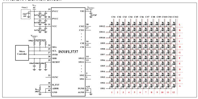
Figure 1 Typical Application Circuit (12×12)
