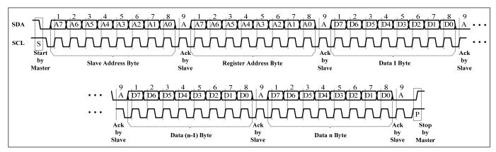
Figure 7 Writing to IS31FL3737 (Automatic address increment)
