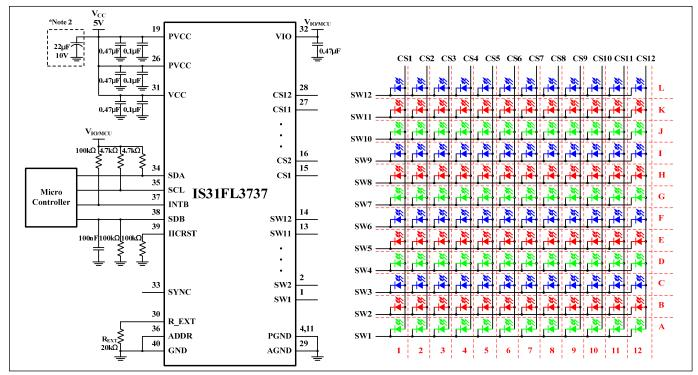
Figure 2 Typical Application Circuit (RGB)
