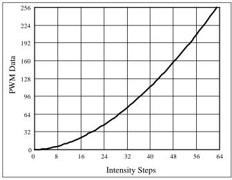
Figure 14 Gamma Correction (64 Steps)
