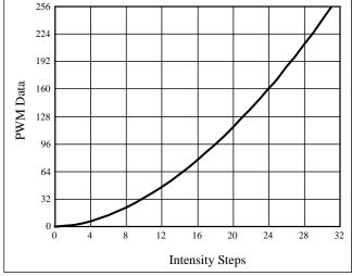
Figure 13 Gamma Correction (32 Steps)
