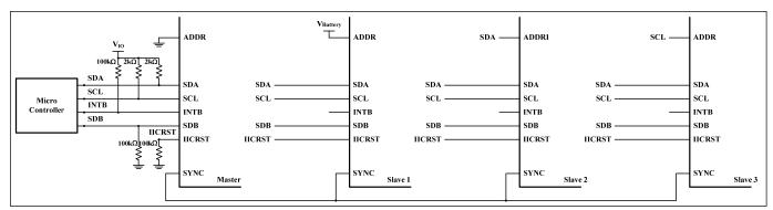
Figure 3 Typical Application Circuit (Four Parts Synchronization-Work)
