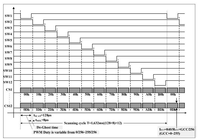
Figure 12 Scanning Timing
