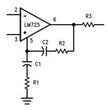
Figure 19. Frequency Compensation Circuit
