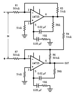
Figure 22. ±100V Common Mode Range Differential Amplifier
