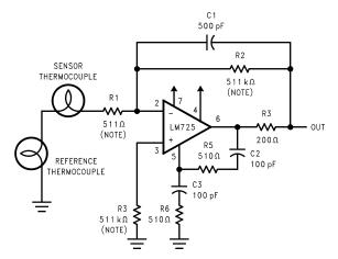
Figure 1. Thermocouple Amplifier
