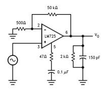
Figure 17. Transient Response Test Circuit
