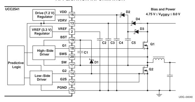
Figure 10. Mode 2 With Common Bias and Power Input Voltages Between 4.75 V and 8.0 V
