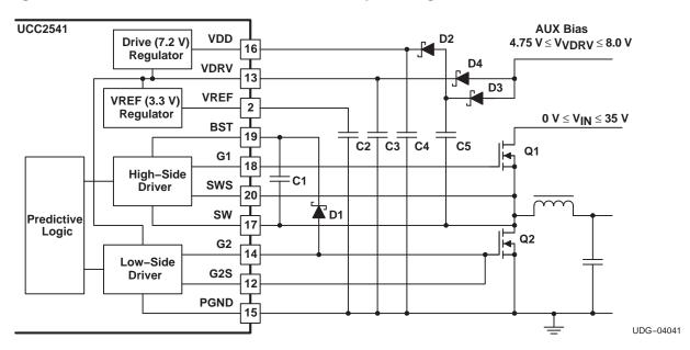
Figure 11. Mode 2 With Separate Power/ Bias (4.75 V and 8.0 V)
