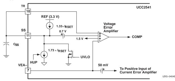
Figure 16. Using the Soft-Start Feature
