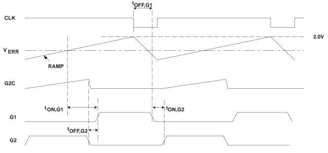
Figure 1. Predictive Gate Drive Timing Diagram
