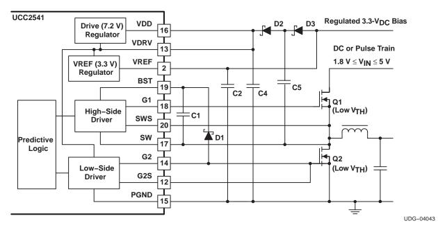
Figure 13. Mode 3 With Regulated 3.3-V<sub>DC</sub> Bias, Low Threshold Power MOSFETs
