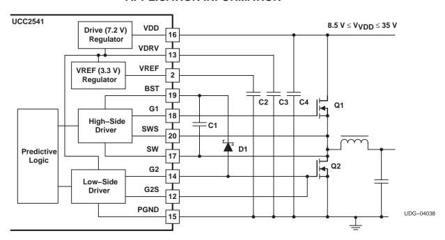
Figure 8. Mode 1 With Combined Power/Bias for Input Voltages Between 8.5 V and 35 V
