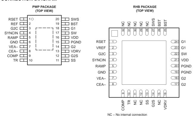
NOTE: The PowerPAD™ is not directly connected to any lead of the package, but is thermally connected to the substrate of the device. The exposed dimension is 1.3 mm x 1.7 mm for the PWP package and 3.25 mm x 3.25 mm for the RHB package. However, the tolerances can be +1.05 mm / -0.05 mm (+41 mils / -2 mils) due to position and mold flow variation.
