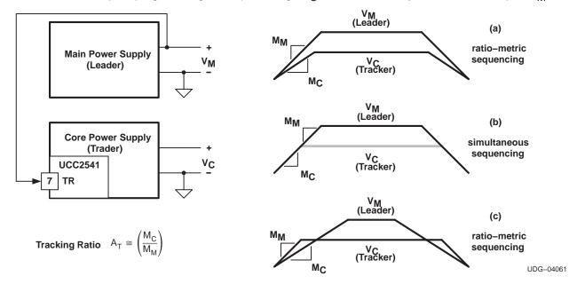
Figure 19. Ratio-Metric Tracking
