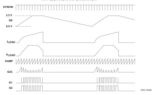
Figure 4. Typical Hiccup Mode waveforms
