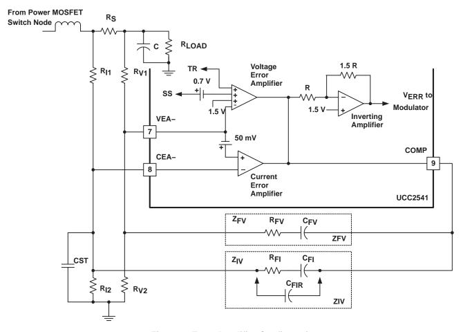
Figure 3. Error Amplifier Configuration
