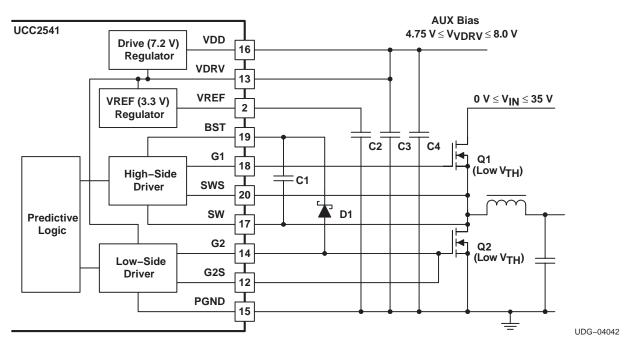
Figure 12. Mode 2 With Auxiliary Biasing for Bias Voltages Between 4.75 V and 8.0 V and Logic Level or Low Threshold Power MOSFET Transistors
