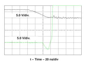
Figure 33. Predictive Gate Drive - G2 Falling
