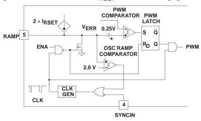
Figure 6. Oscillator and PWM Modulator
