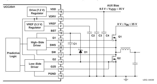
Figure 9. Mode 1 With Separate Power/ Bias Voltages Between 8.5 V and 35 V
