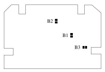
Fig.3 - Solder Bridge Link Selection Of Input Range
