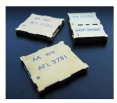
Filter with printed wire board cover
