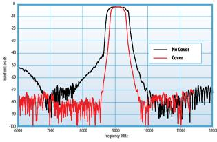
**High K substrate provides Higher Field** Confinement – 9 GHz Filter (30 mil CF with and without cover).
