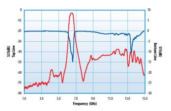
Thin Film - 10GHz 4 Pole Band Pass with Bandstop Filter
