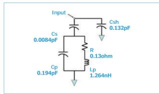
over resonant frequency, coupling and input impedance. The structure also provides an integrated DC blocking function, thus eliminating a tolerance sensitive element from the bill of materials. For wide bandwidth circuit modeling, S-Parameters are recommended. S-Parameters are available for downloading from our website (www.dilabs.com). The resonators are readily customized for frequency, coupling, Q, tunability and assembly requirements.
