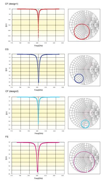
DLI resonators are direct in frequency. So in addition to all of the other benefits no multiplication is required as there would be in other technologies. As a solid block of ceramic they are also non microphonic
