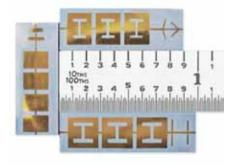
6.5 GHz Symmetric Dual Mode Bandpass Filter
