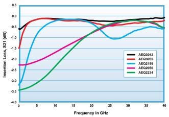
Excellent, repeatable microwave performance is achieved by application of precision thin film fabrication and DLI Hi-K Ceramic materials. DLI's unique design solution provides near Ideal R-C frequency response, far superior to "Stacked R-C chip" Assemblies.
