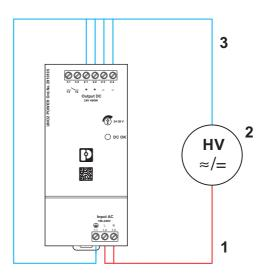
Figure 1 Potential-related wiring for the high-voltage test
