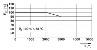
Figure 28 Output power depending on the installation height
