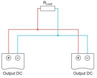
Figure 25 Schematic diagram, power increase in parallel operation
