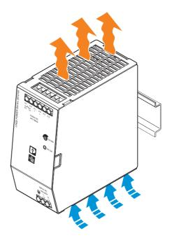
Figure 7 Schematic diagram of the convection cooling
