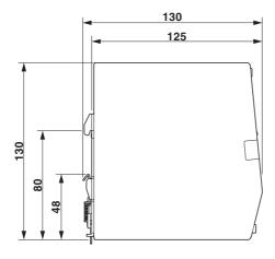
Figure 6 Device dimensions (dimensions in mm)
