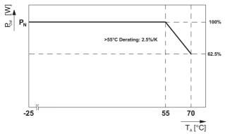
Figure 27 Output power depending on the ambient temperature
