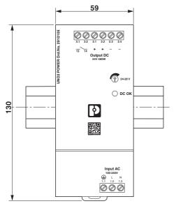
Figure 5 Device dimensions (dimensions in mm)
