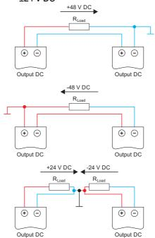
Figure 24 Schematic diagram, power increase in series operation
