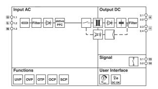
Figure 4 Block diagram
