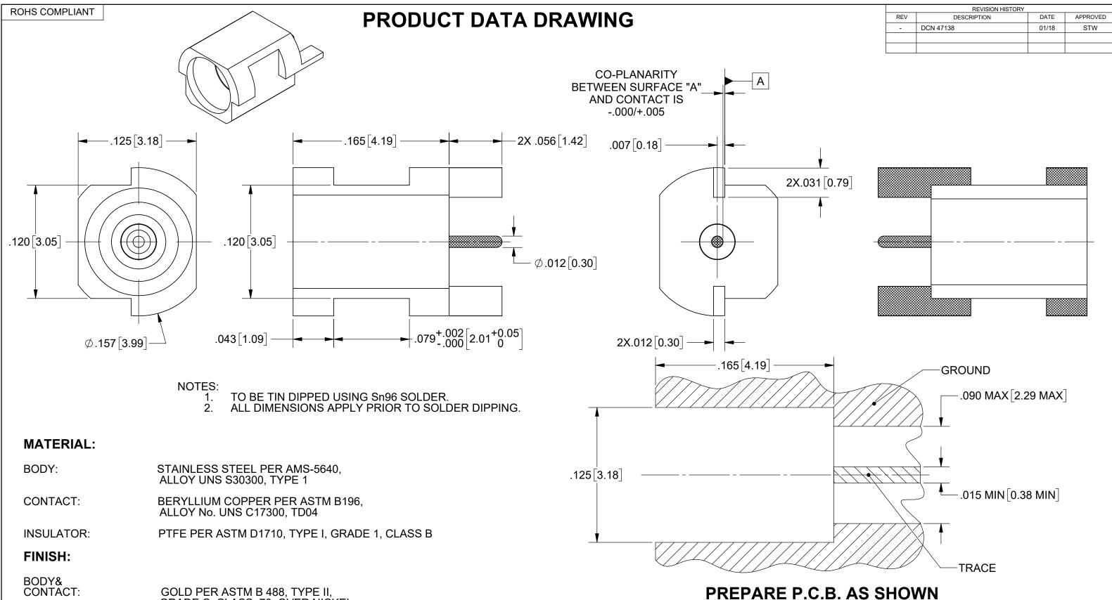
GOLD PER ASTM B 488, TYPE II, GRADE C, CLASS .76, OVER NICKEL CONTACT: PER AMS-QQ-N-290, CLASS 1.
