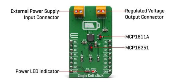
MCP16251 that's featured on Single Cell Click operates and consumes less than 14  $\mu$ A from battery after start-up, while operating at no load. The device provide a true disconnect from input to output while in shutdown EN = LOW. While in shutdown it consume les than 0.6  $\mu$ A from battery.
