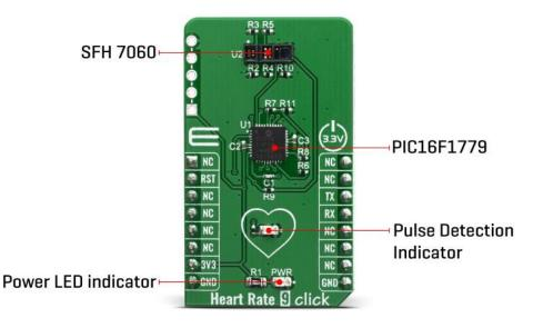
This Heart Rate 9 Click board<sup>™</sup> introduces Microchip's proprietary method (hereafter "proprietary method") of measuring multiple signals in a body using pseudorandom binary sequence generation and phase division multiplexing. This proprietary method uses a special encoding/decoding scheme to allow multiple light-emitting diodes (LED) transmitting light simultaneously with a single photodiode to condition each light from the combined lights at the receiving side.
