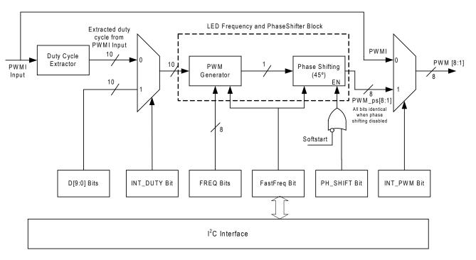
Figure 1— LED PWM Dimming Control
