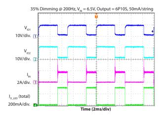
LED Dimming Without Phase Shift
