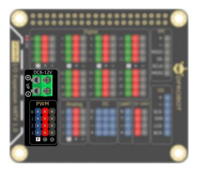
• IIC Port: IO expansion board has 3 groups of IIC ports that are led out via Raspberry Pi GPIO2 (SDA.1) and GPIO3 (SCL.1) (BCM code). IIC Learning Guide.
