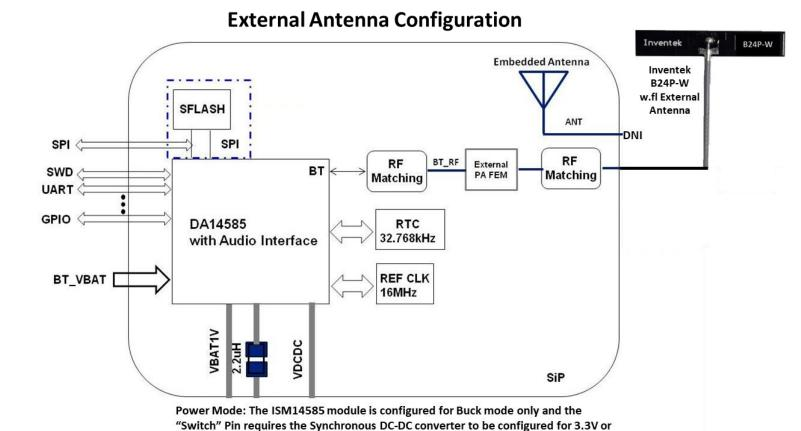
Figure 2 Inventek ISM14585-L35 SiP Block Diagram
