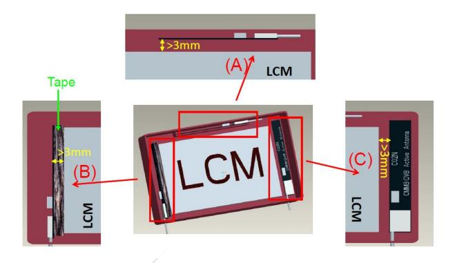
When there are metal objects on the sides of the PCB antenna, make sure to keep a distance of 3mm from one end and 5mm from another end:
