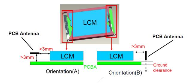
Another option is to make a rib or fixture to locate the PCB antenna on the side of the unit, to simplify production:
