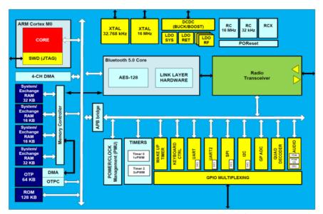
Figure 1 Dialog DA14585 SoC Block Diagram
