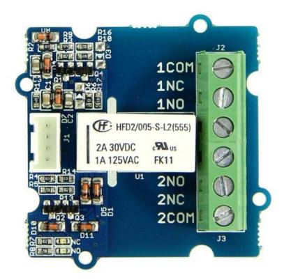
This module is based on 2-Coil Latching Relay. Contrast to the ordinary relay, this latching relay does not need continuous power to keep the state, only a rising/falling pulse is needed to change the work state. Even the power can be removed when the work state do not need to change, making this module especially suitable for low-power projects.
