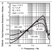
Figure 17. Total Harmonic Distortion + Noise vs Frequency
