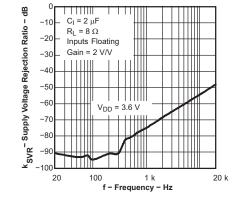
Figure 25. Supply Voltage Rejection Ratio vs Frequency 25
