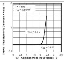
Figure 23. Total Harmonic Distortion + Noise vs Common Mode Input Voltage
