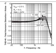
Figure 22. Total Harmonic Distortion + Noise vs Frequency
