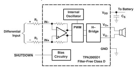
Figure 40. Typical TPA2005D1 Differential Input for a Wireless Phone
