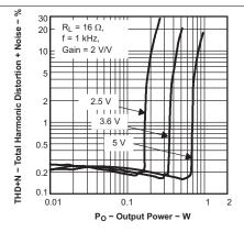
Figure 15. Total Harmonic Distortion + Noise vs Output Power
