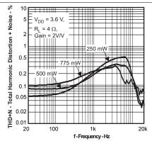
Figure 21. Total Harmonic Distortion + Noise vs Frequency
