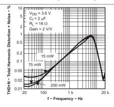
Figure 19. Total Harmonic Distortion + Noise vs Frequency
