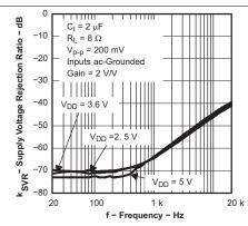
Figure 24. Supply Voltage Rejection Ratio vs Frequency
