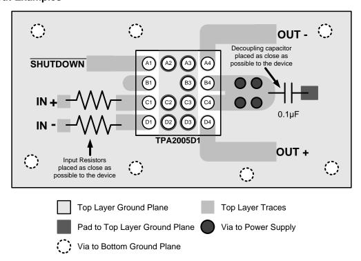
Figure 45. TPA2005D1 MicroStar Junior™ BGA Package Layout Example
