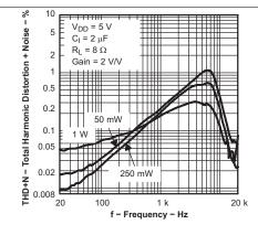
Figure 16. Total Harmonic Distortion + Noise vs Frequency
