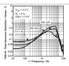
Figure 20. Total Harmonic Distortion + Noise vs Frequency
