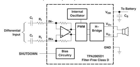
Figure 42. TPA2005D1 Differential Input and Input Capacitors
