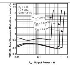
Figure 13. Total Harmonic Distortion + Noise vs Output Power
