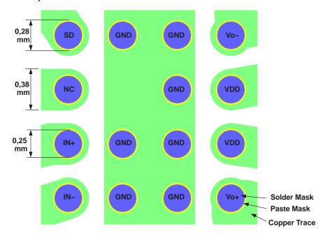
Figure 44. TPA2005D1 MicroStar Junior BGA Board Layout (Top View)
