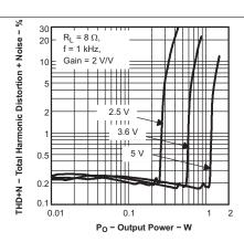
Figure 14. Total Harmonic Distortion + Noise vs Output Power
