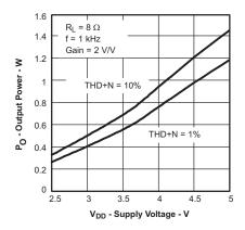
Figure 41. Output Power vs Supply Voltage
