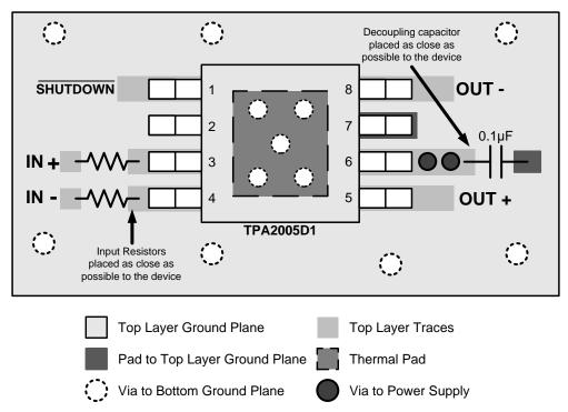
Figure 47. TPA2005D1 DGN Package Layout Example
