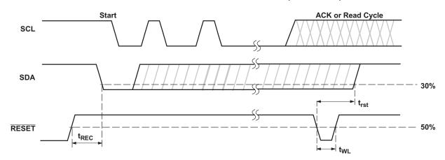
Figure 2. Reset Timing
