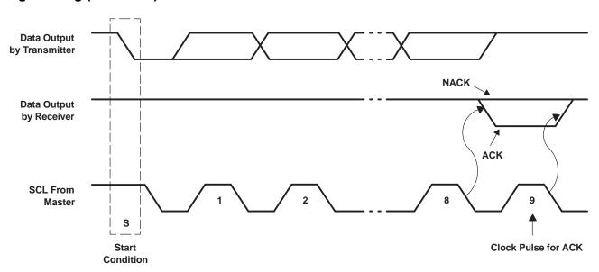
Figure 7. Acknowledgment on the I<sup>2</sup>C Bus
