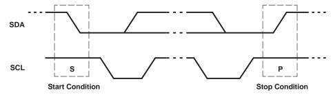
Figure 5. Definition of Start and Stop Conditions
