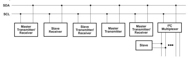
Figure 6. System Configuration
