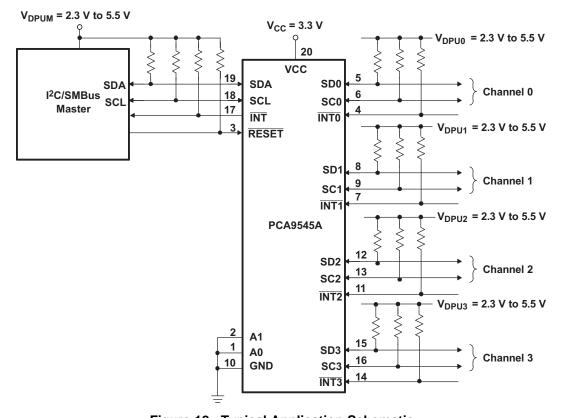
Figure 12. Typical Application Schematic
