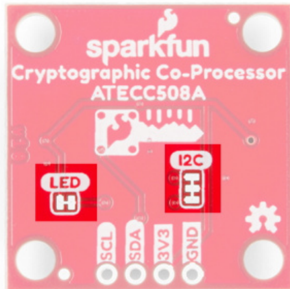
LED and I2C jumper pads.
