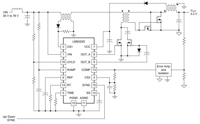
Figure 14. Simplified Active Clamp Forward Power Converter
