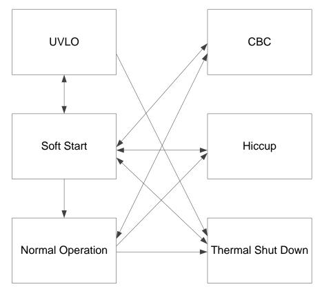
Figure 13. Functional Mode Transition Diagram
