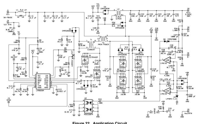
Figure 22. Application Circuit
