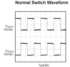
Input/Output Waveform Negative Pulse
