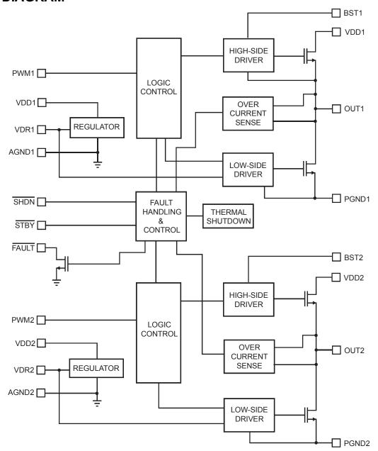
Figure 2—Function Block Diagram
