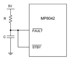
Figure 1— Fault Protection Circuit
