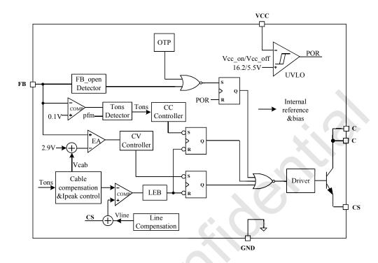
Figure 4.1: FT839NX Block Diagram
