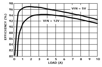
FIGURE 7. EFFICIENCY vs LOAD CURRENT (V<sub>OUT</sub> = 3.3V)
