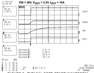
FIGURE 9. TYPICAL SOFT-START WAVEFORM
