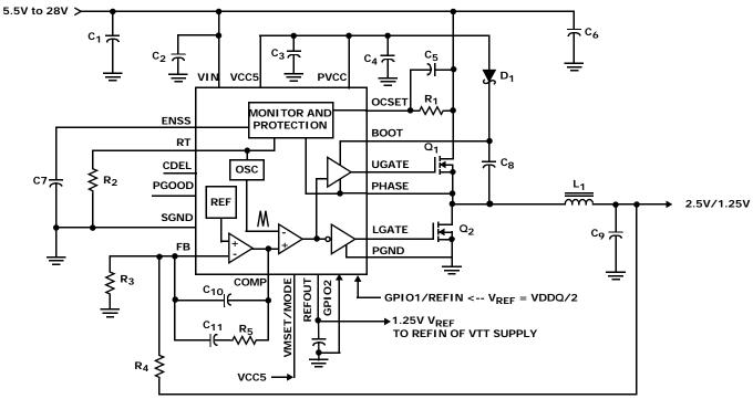
CONFIGURATION FOR DDR TERMINATION/EXTERNALLY REFERENCED TRACKING APPLICATIONS
