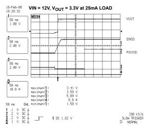
FIGURE 14. PREBIASED OUTPUT AT 25mA LOAD
