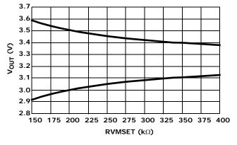
FIGURE 11. VOLTAGE MARGINING vs. VMSET RESISTANCE
