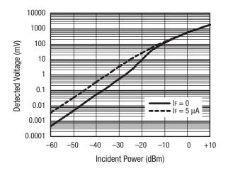
Figure 7. Detector Voltage @ 2.45 GHz (100 k $\Omega$  Video Resistance)
