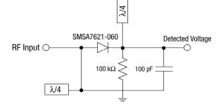
Figure 2. Schematic of a 24 GHz Detector Design
