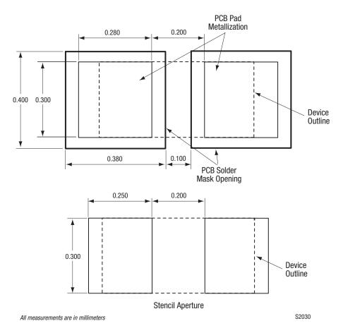
Figure 10. SMSA7621-060 PCB Layout Footprint
