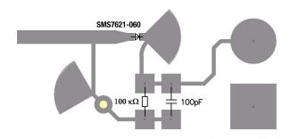
Figure 3. Layout for a 24 GHz Detector Design
