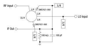
Figure 4. Schematic of a 24 GHz Rat-Race Mixer
