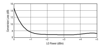
Figure 9. Conversion Loss vs LO Power
