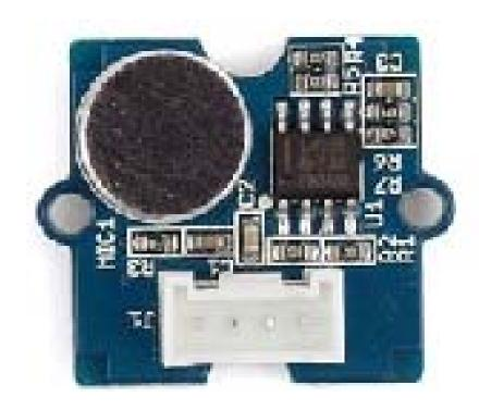
Grove - Sound Sensor can detect the sound intensity of the environment. The main component of the module is a simple microphone, which is based on the LM386 amplifier and an electret microphone. This module's output is analog and can be easily sampled and tested by a Seeeduino.
