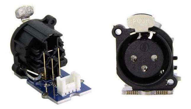
The Grove – DMX512 is a adapter from Grove interface to DMX512 interface(industry standard EIA-485 interface. The module is based on SN75176 chip which can balance transmission lines and meet ANSI Standard EIA-485 interface. Now it is convenience to control stage lighting and DMX512 console for Arduino.
