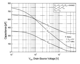
Figure 5. Capacitance Characteristics
