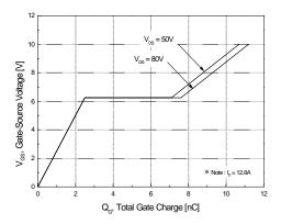
Figure 6. Gate Charge Characteristics
