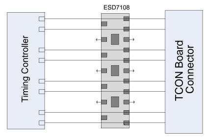
Figure 6. V-by-One HS Layout Diagram (for LCD Panel)
