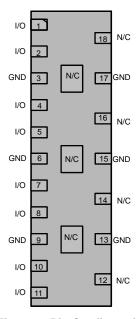
Figure 2. Pin Configuration
