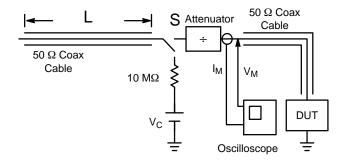
Figure 3. Simplified Schematic of a Typical TLP System
