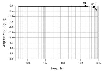
Figure 5. ESD7108 Insertion Loss
