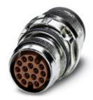
Device connector, front mounting, straight, SPEEDCON locking, M17, Number of positions: 17, Type of contact: Male connector, Crimp connection, Axial O-ring, Central fixing, shielded: yes
